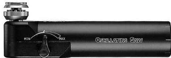
The attachment can be locked in eight different positions. When the attachment needs to be rotated after it is coupled, it must first be uncoupled, and the attachment is pulled approx. 1 cm forward. Adjust the desired angle (45° increments), and shove the attachment back toward the tool until it locks into place.
